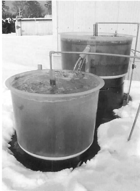
Fig. 1 A kelp-abalone culture system in which warmed deep-sea water ( 14^{\circ}\text{C} ) is reused in the lower tank to rear abalone after used for growing kelp ( Saccharina japonica ) in the upper tank. Abalones were fed the blade of cultured kelp as well as attached diatoms growing inside the abalone tank. 加温深層水をかけ流した上側の水槽でマコンブを培養し、その排水を利用して下側の水槽でアワビを飼育する養殖システム。
